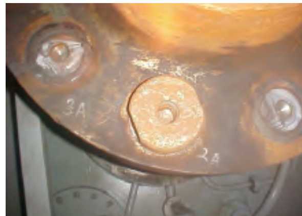
Example of the problems that can occur using shrink fit bolts
