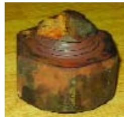
Traditional shrink fit bolts are manufactured with an outer diameter that is larger than the coupling hole. This means they first have to be frozen in liquid NO<sub>2</sub> or dry ice and alcohol until the outer diameter reduces sufficiently to allow the bolt to be inserted in the hole.
