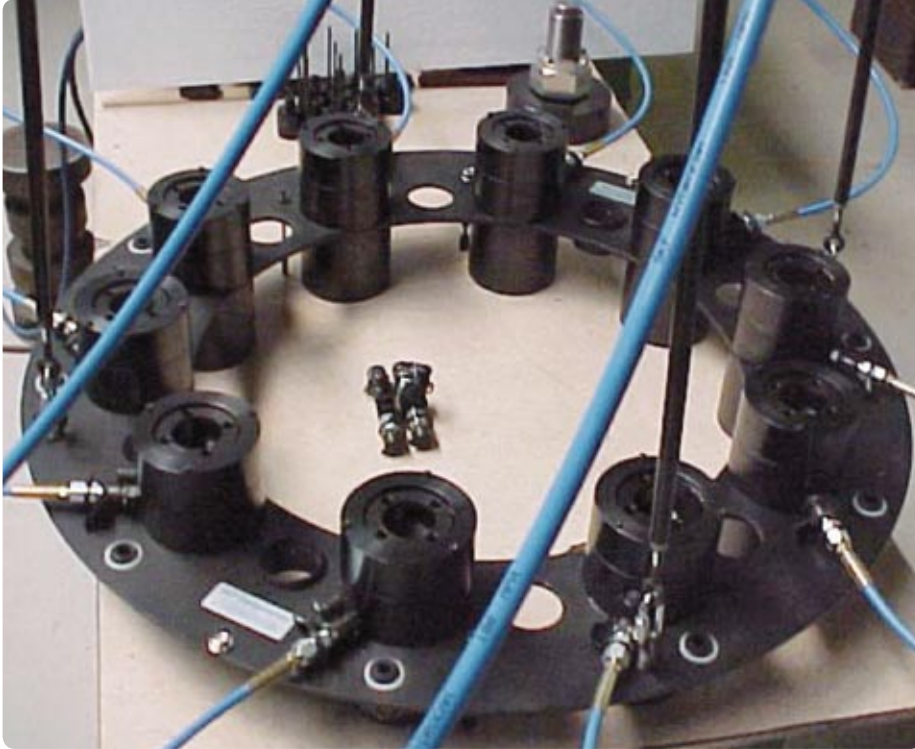
Example of tool for semi-simultaneous tightening (50%) of cover head on a chemical vessel
