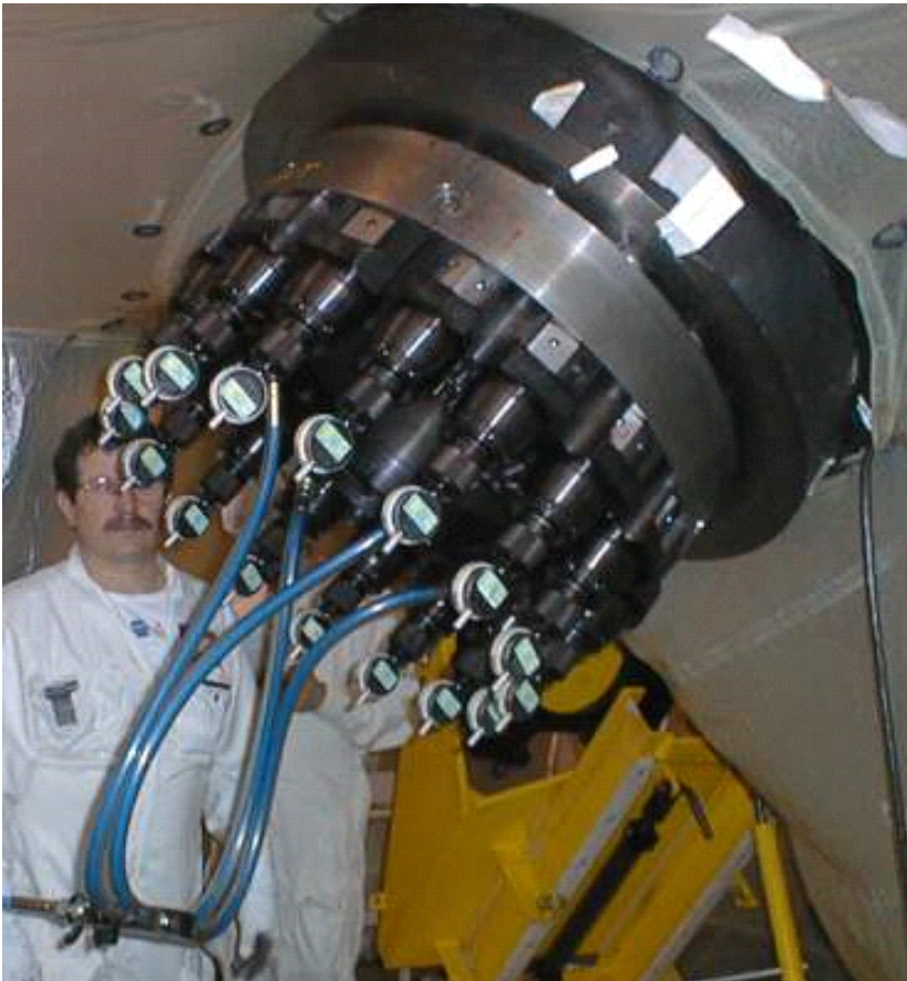
Segmented Ring Tensioning Unit for Primary / Secondary Manway of a Steam Generator
