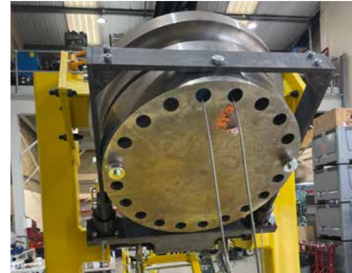
SG Manway Cover Test Rig
