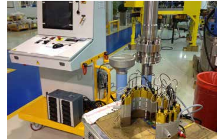
Control Rod Drive Mechanism Tensioner being Tested
