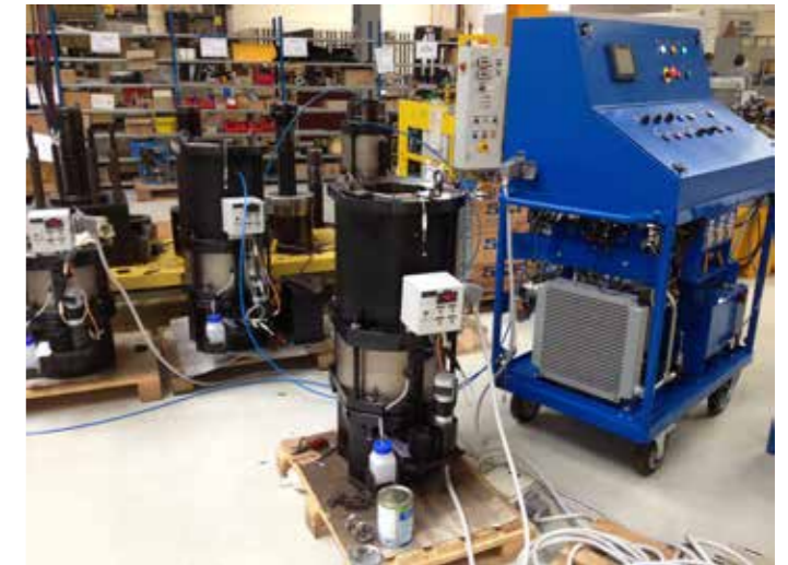
Segmented Tensioning Rig on Control Panel
