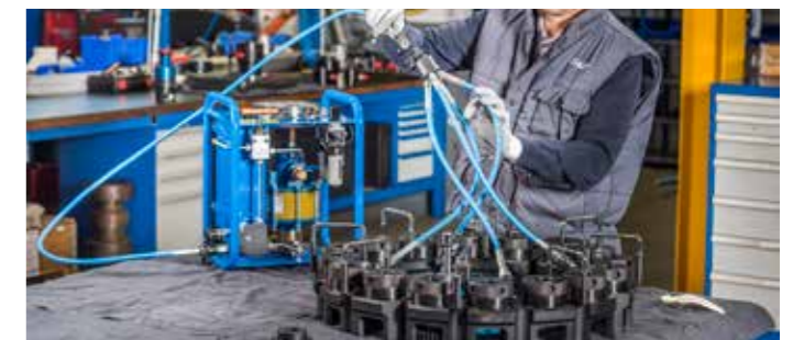
Tensioning Rig being Tested
