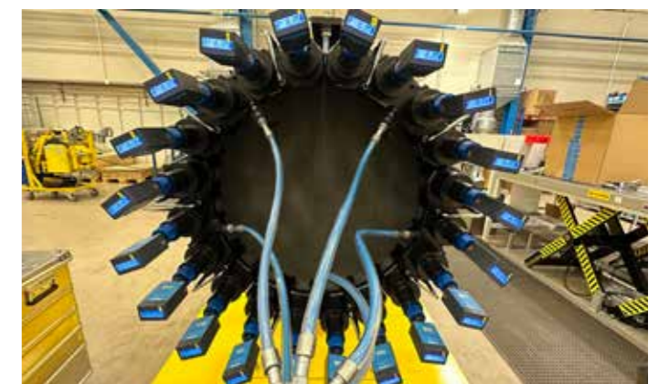
Segmented Tensioning Rig on Test with Bluetooth Sensors
